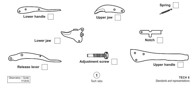
**4.** Grip the pliers with one hand. Gently squeeze the lower handle and observe what happens to the spring. Then, release the pressure.
