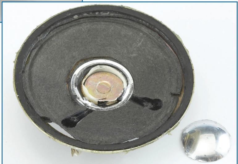
2. Cut the speaker cone in two with the retractable utility knife. One section will remain attached by wires.
