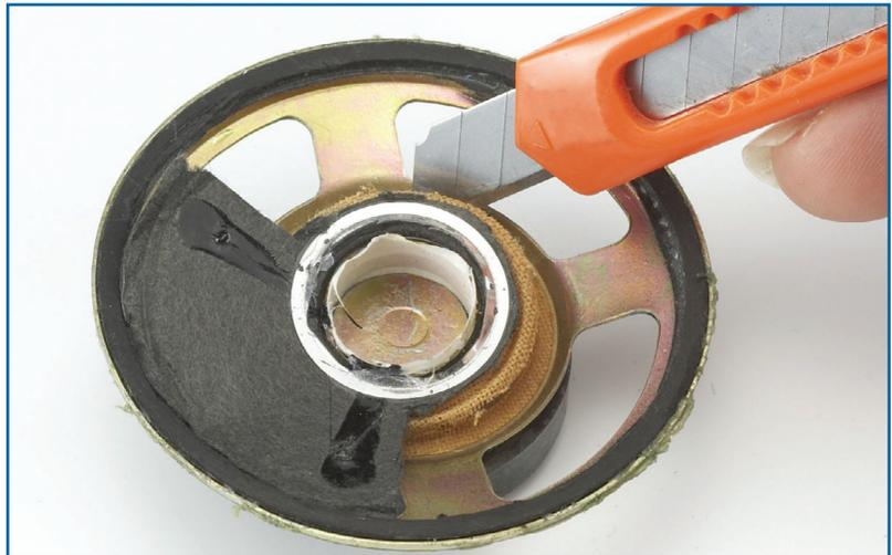
5. Remove the coil from the magnetic slot.
