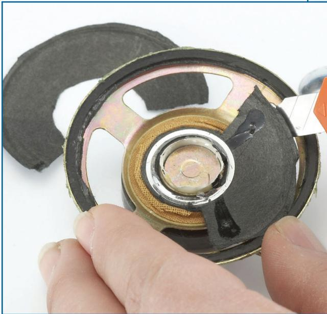
3. Cut the support insulating the speaker wires with the retractable utility knife.
