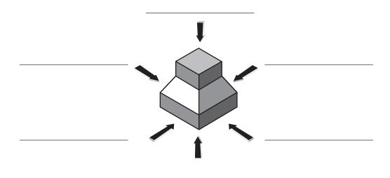
2. The drawing below shows the three views generally illustrated in a multiview projection. Write the name of each of these views in its appropriate space.
