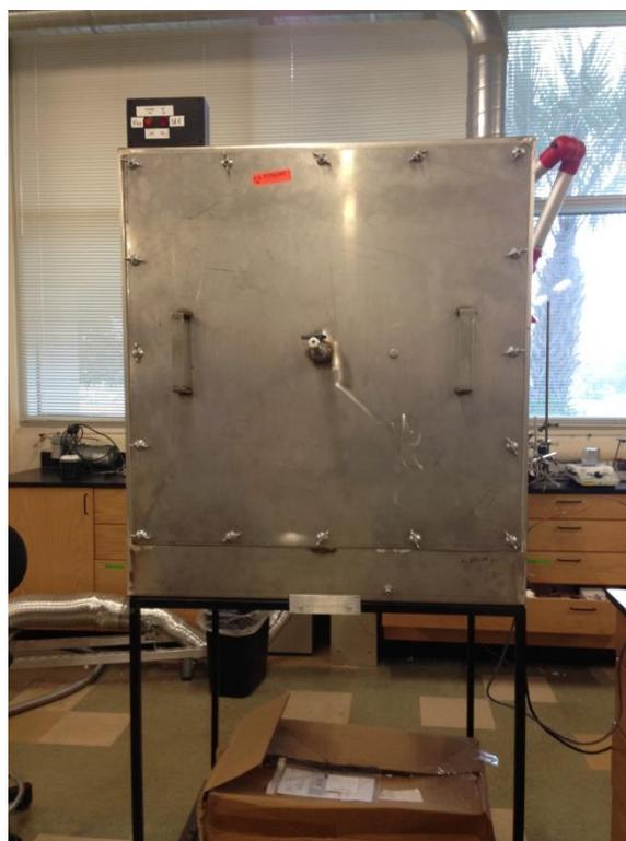
Figure 4. Photograph of stainless steel chamber having an internal volume of 604 liters.
