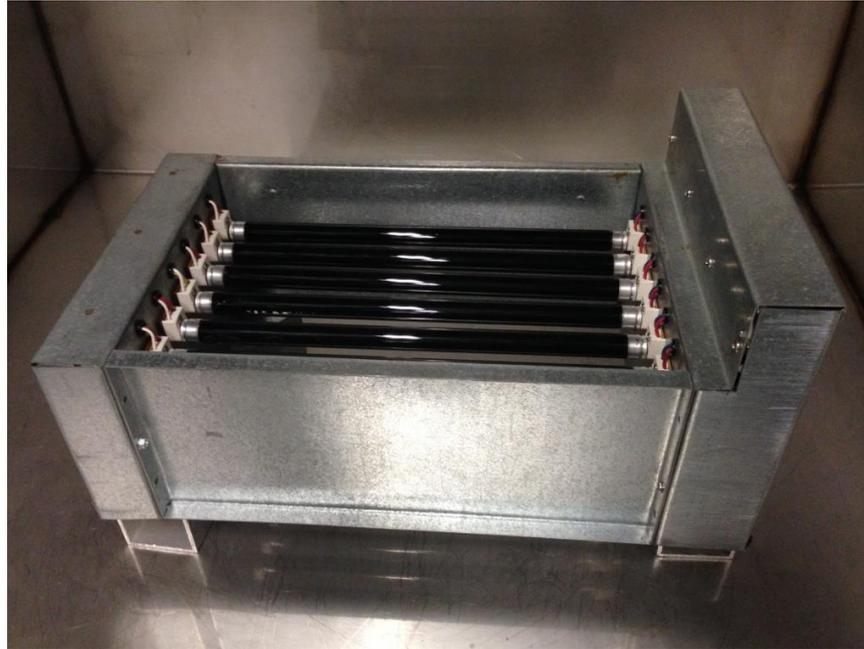
Figure 1. Photograph of photo-electrochemical air purifier showing six UV lamps at the base of the system.
