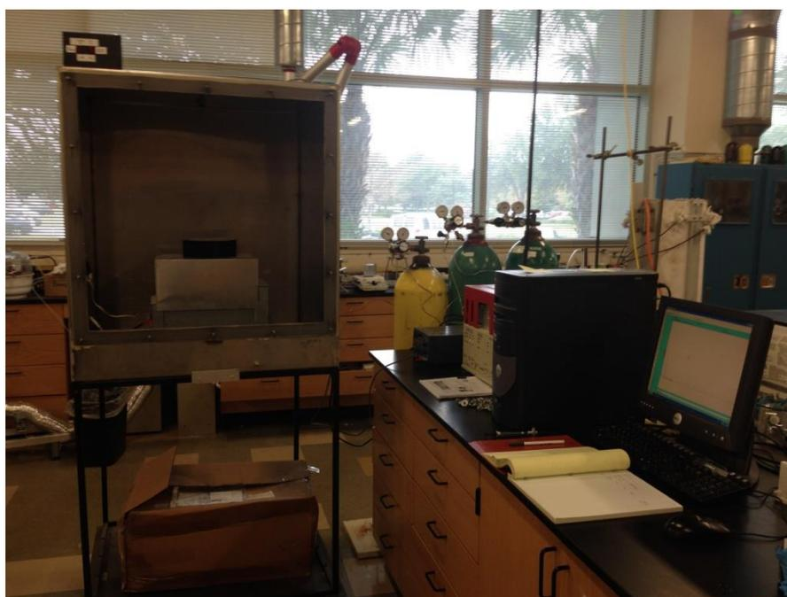
Figure 6. Photograph of test setup showing stainless steel chamber with photo-electrochemical air purifier inside, GC-FID and computer.
