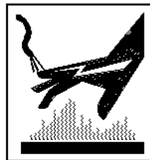
High Voltage & Hot Surface
