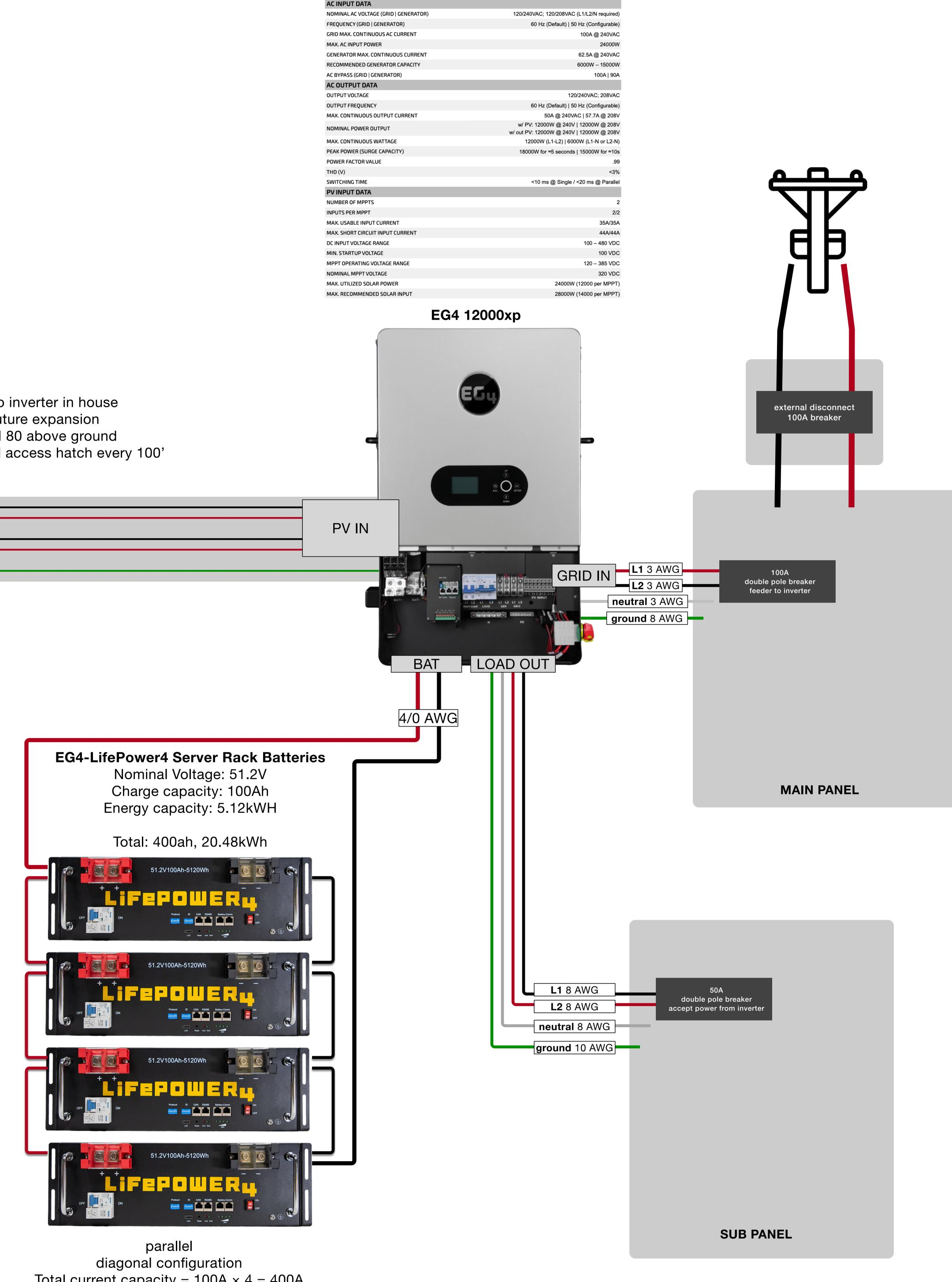
Total current capacity =  $100A \times 4 = 400A$ Voltage remains at 51.2V
