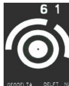
Figure 11 (below): Signalled ground control point (coded bar mark for automatic measurement of image coordinates)
