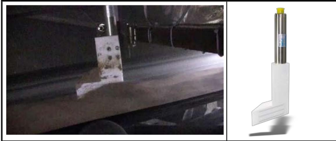
Image: SONO-MOVE PTFE probe above a conveyor belt deployed for the measuring of adhesive limestone sand.
