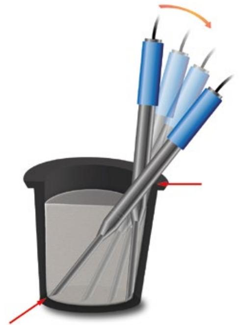
Fig. 5: Measuring procedure for concretes softer than F3
