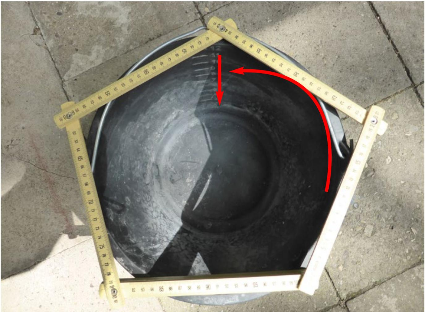
Fig. 3: Rotating the bucket by approx. 20 cm after taking each measurement
