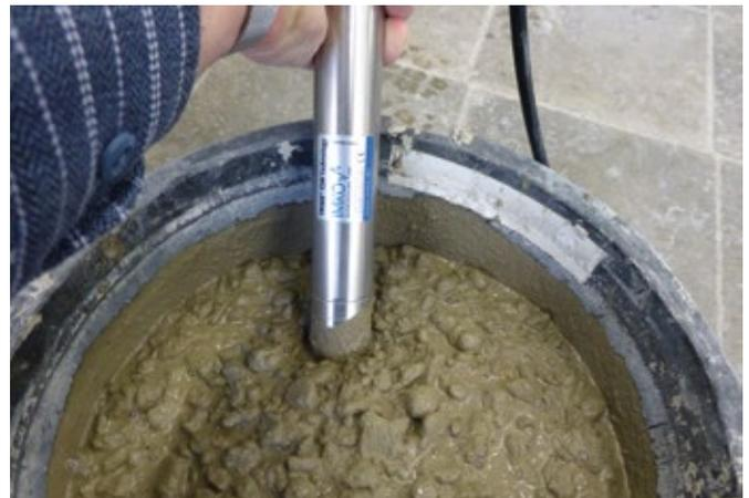
Figs. 1,2: Carrying out the measuring procedure using the Sono WZ (radar impulse technology) with a fresh concrete sample
