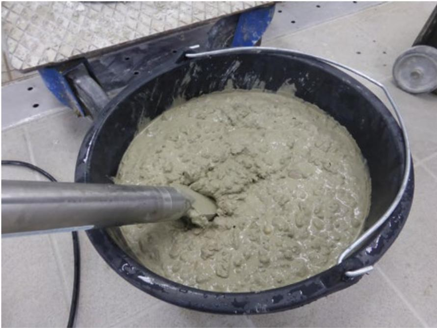
Fig. 4: Particular care must be taken that the measuring sensor is entirely moistened with concretes with great ultra-fine content or low water content.
