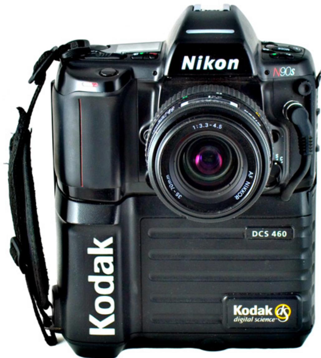
The Kodak DCS 460 was introduced in 1995. At the time, it was the highest resolution digital camera in the world- at 6.2 megapixels. It cost a whopping- $35,600 USD
