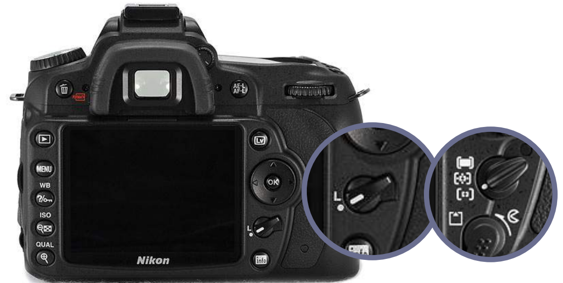
Some Nikon cameras can move the spot meter point using this dial on the rear of the camera.
