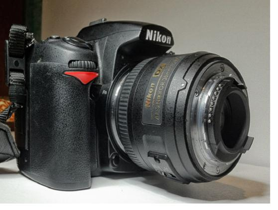
A reversed lens generally works best with a prime lens (not a zoom). However, they can be used with some zoom lenses as well. Another way to get a zoom lens to close-focus is by using a device called extension tubes. Extension tubes insert between the lens and the camera body.
