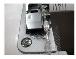
TIP: Hold onto them in the back of the foot as you are placing the foot back into the machine so the bead strand doesn't fall out.
