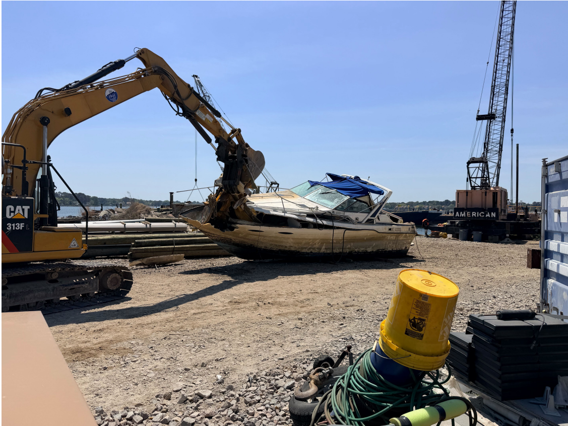
An image of an ADV removed from the Elizabeth River and crushed for disposal. Photo Credit: BoatUS Foundation
