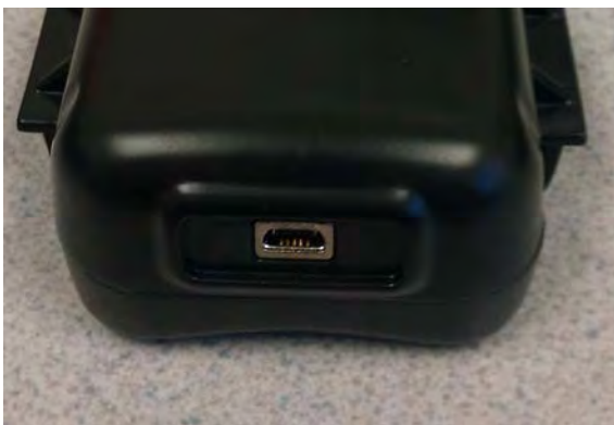
Figure 4. UniTrak II USB Power Adapter. The UniTrak II features a new USB power adapter for conveniently charging the unit while in residence, away from the residence, or traveling in a vehicle.
