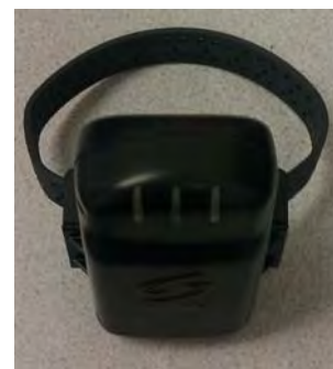
The UniTrak One-Piece GPS Tracking Unit utilizes a dual radio frequency design to ensure reliable monitoring.
