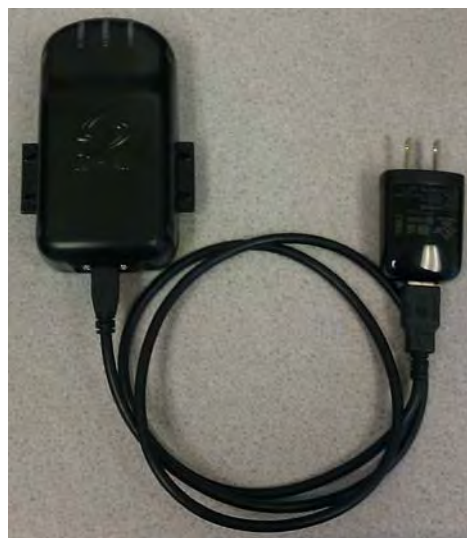
Figure 4. UniTrak II USB Power Adapter. The UniTrak II features a new USB power adapter for conveniently charging the unit while in residence, away from the residence, or traveling in a vehicle.
