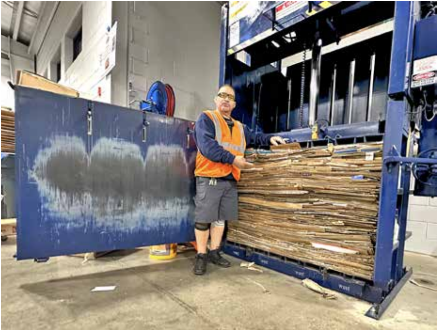
City employee Ramon Rodriguez explains the baler to me. Each bale of cardboard is worth $100 - $150! Making this, the paper shredder, and metal salvage profitable. Returning needed money to the general funds.
