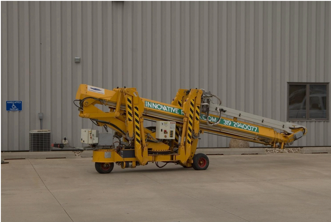
Wheel atrium manlift in stowed position
