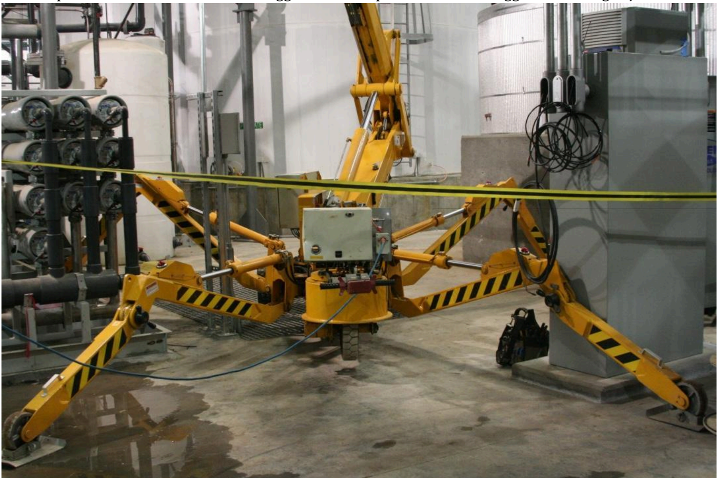
Can morph to most situations. Each outrigger has three positions and outriggers have hinged joints.
