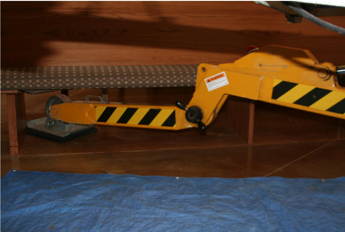
Outrigger with hinged joints
