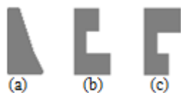
Figure 2 Different soil profiles considered (a) linearly increasing profile (b) Varied profile I and (c) Varied profile II
