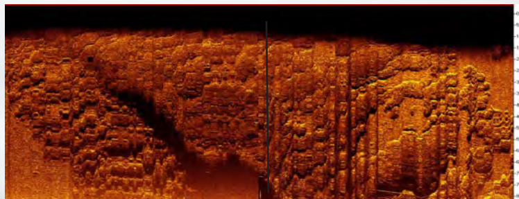
Motion Tolerant Mode Sonar example: During turbulent conditions, the data on the left of side of this image was recorded using the EdgeTech 4205 Motion Tolerant mode. The right side of the image, depicting motion induced striping was captured without the Motion Tolerant mode for comparison.
