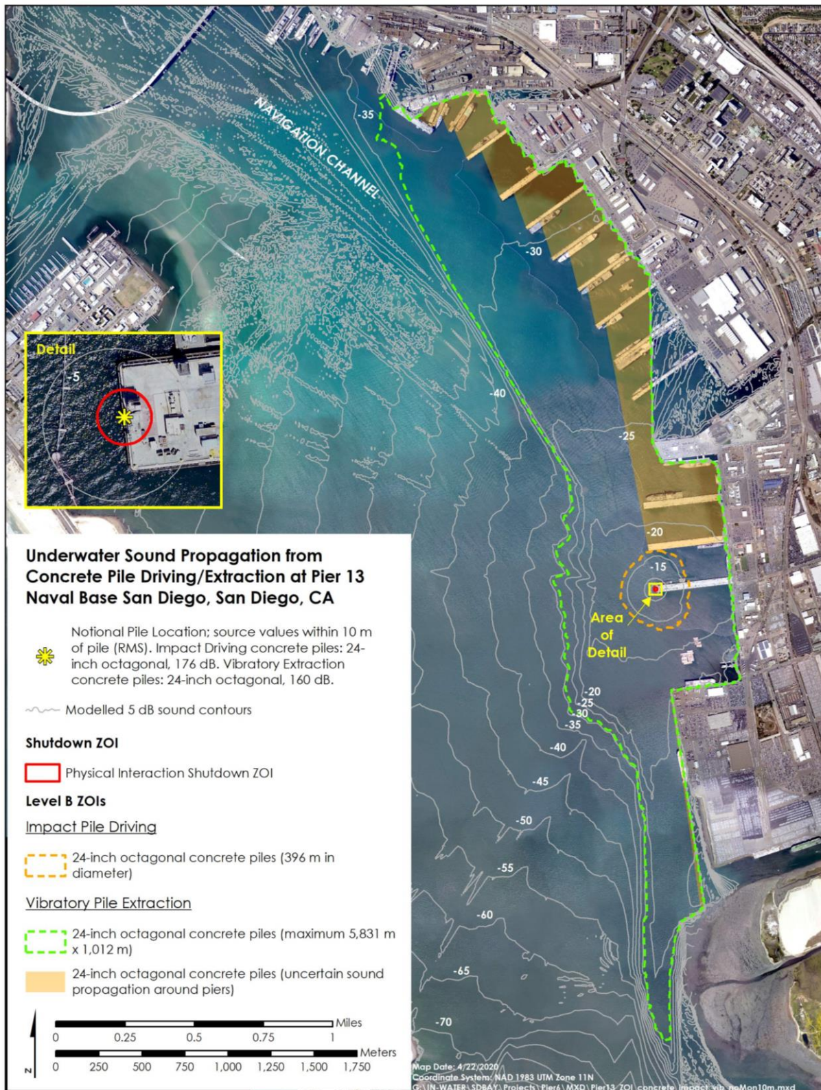
Figure 3-11. Level B ZOIs for impact driving and vibratory extraction of 24-inch octagonal concrete piles based on modeled TL for a representative southern area location at NBSD (Pier 13).
