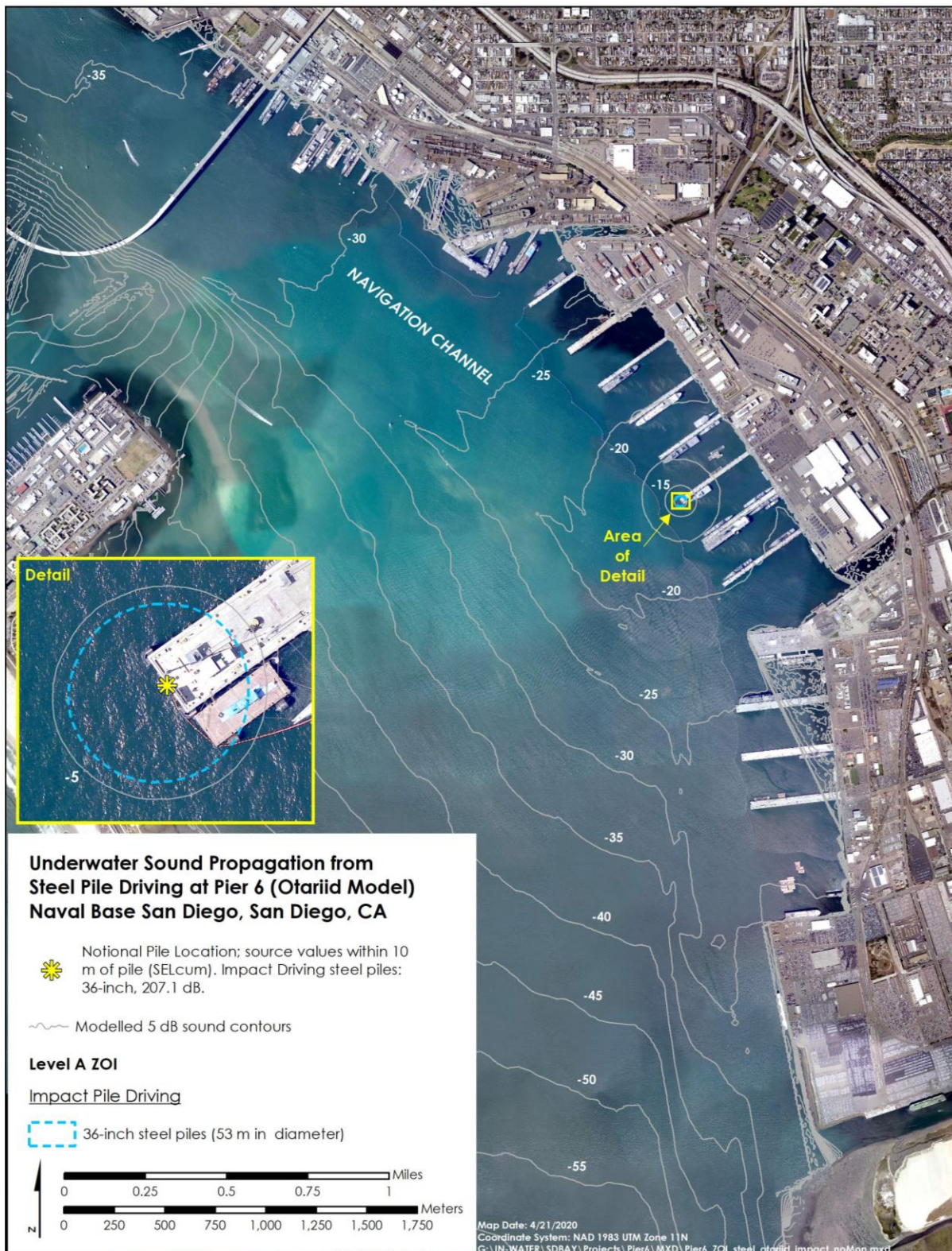
Figure 3-5. Otariid FHG Level A ZOI for impact driving of 36-inch steel piles based on modeled TL for a representative central area location at NBSD (Pier 6).
