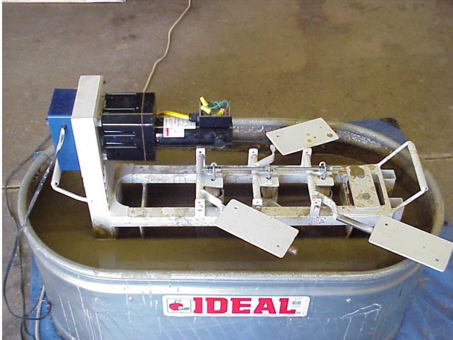
Figure 6, Rotary Abrasion Tester in Drilling Mud Bath
