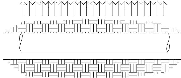
Figure 1, Bearing Force Resulting from Weight
