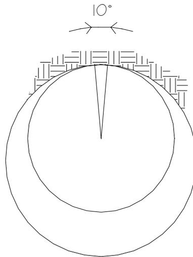
Figure 3, Assumed Bearing Arc
