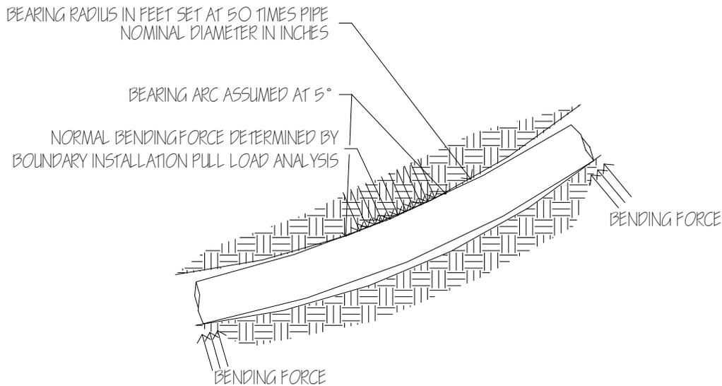
Figure 2, Bearing Force Resulting from Bending
