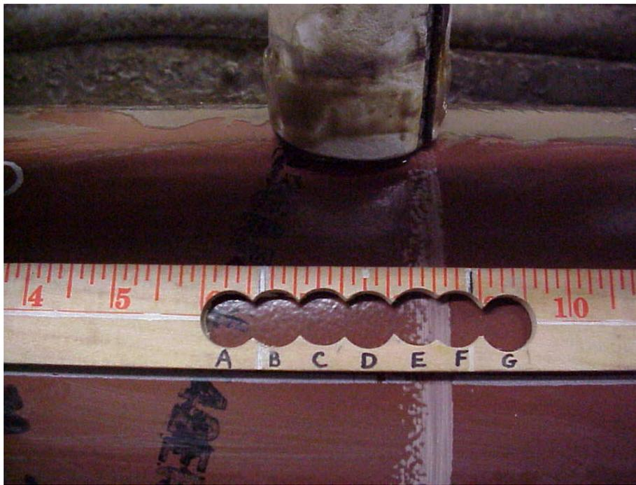
Figure 7, Template with measurement points
