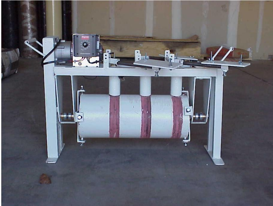
Figure 4, Rotary Abrasion Tester
