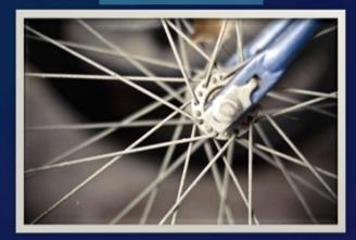
"Tension between the hub and rim is applied evenly in all directions, making the assembly extraordinarily strong and also somewhat flexible and resistant to shock. This uniformly applied tension is what supports your weight on the wheels."
