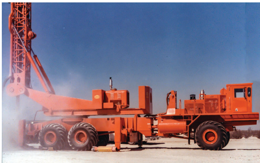
▲ 1978 3000 on Foremost Commander for air drilling in Saudi Arabia.
