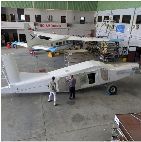
A big project over the last year was the total stripping and repainting of one of our PC-6 airplanes. Also, the Caravan in the background received a whole new avionics upgrade.
