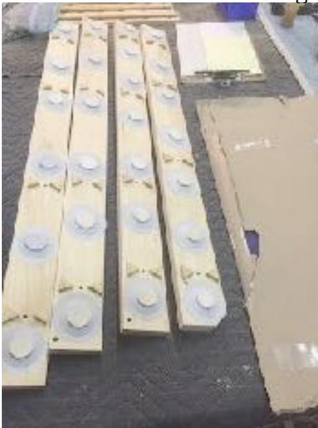
Completed offset pouch boards. These actions control the larger pipes in the instrument.
