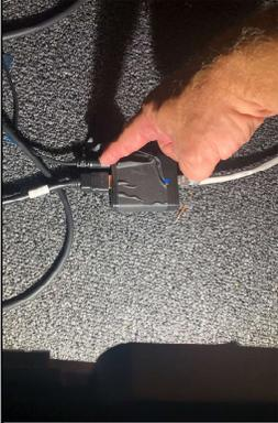
4. Disconnect the power cable from the Video Processor controlling the two disconnected video processors.
