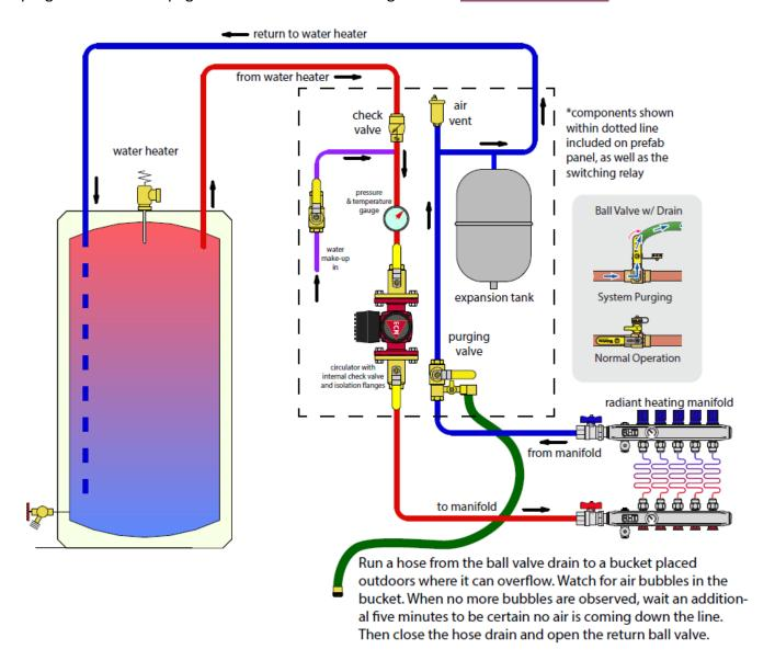
**11. Zone Purging:** When no more air bubbles are observed, wait an additional five minutes to be certain no air is coming down the line. Once there is no more air in each zone, close the corresponding return ball valve and move onto purging the next zone until all zones are purged. The glycol pump will turn off automatically when you close the hose valve. It's crucial to keep the glycol fill plugged in and connected, as it is responsible for maintaining pressure within your system.
