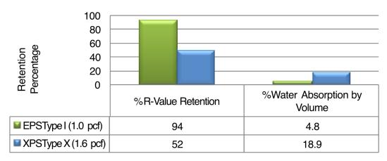
The results demonstrate that EPS Type I outperforms XPS Type X in both R-value retention and decreased water absorption. Further, whereas the in-service R-value of the XPS insulation is reduced by half, expanded polystyrene still delivers 94% of its specified R-value of 3.6 per inch after 15 years. These long term performance advantages make EPS insulation a preferred choice when compared to its competition.
