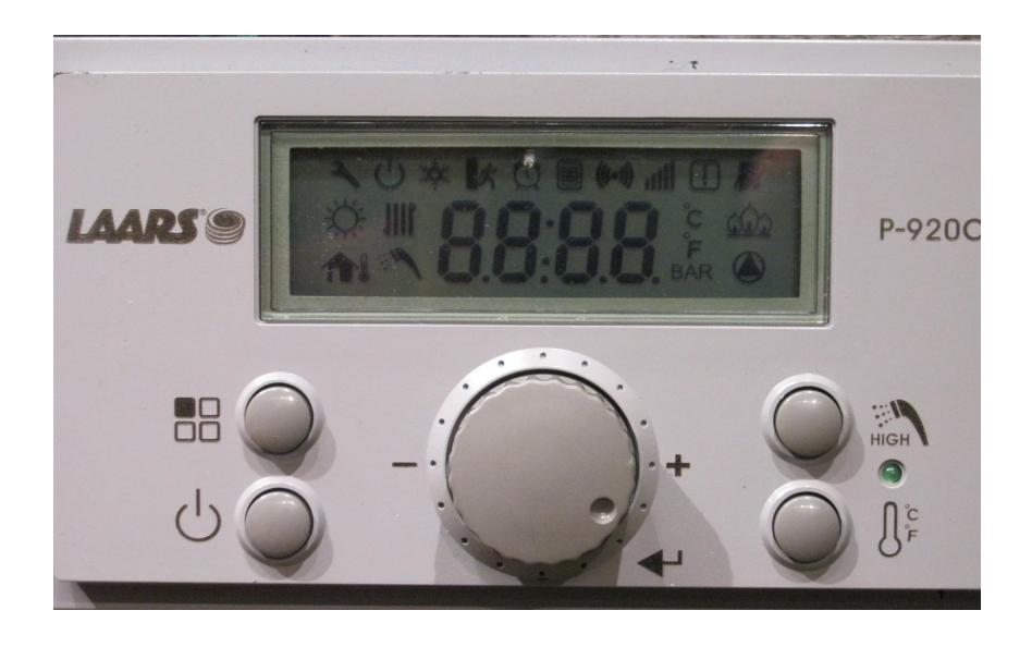
When the unit is powered up the display shows all Icons and runs through a series of numeric codes.
