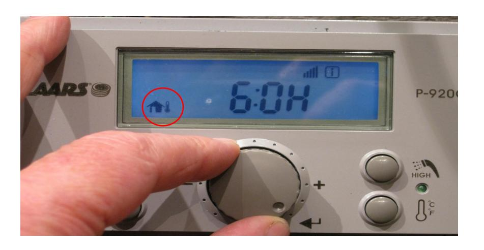
You will see the Out Door Icon when the sensor is connected. Using the Scroll/Select Button locate 6:OH This is the Maximum Out Door Temperature then press the select button
