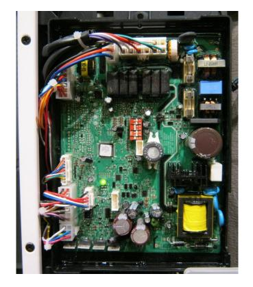
CO2 adjustment are made when the boiler is in "Min Fire" so with the Display Powered **OFF** set DIP Switch #7 to the **ON** position to run boiler in "Min Fire"
