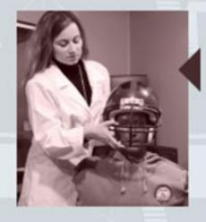
Football helmets are designed to protect players' heads, not their hearing. Openings on either side of the helmet allow them to hear crowd noise and calls on the field. When Oticon audiologists measured sound levels with a regulation helmet using KEMAR, an acoustic research mannequin, sound levels were virtually the same with and without the helmet.
