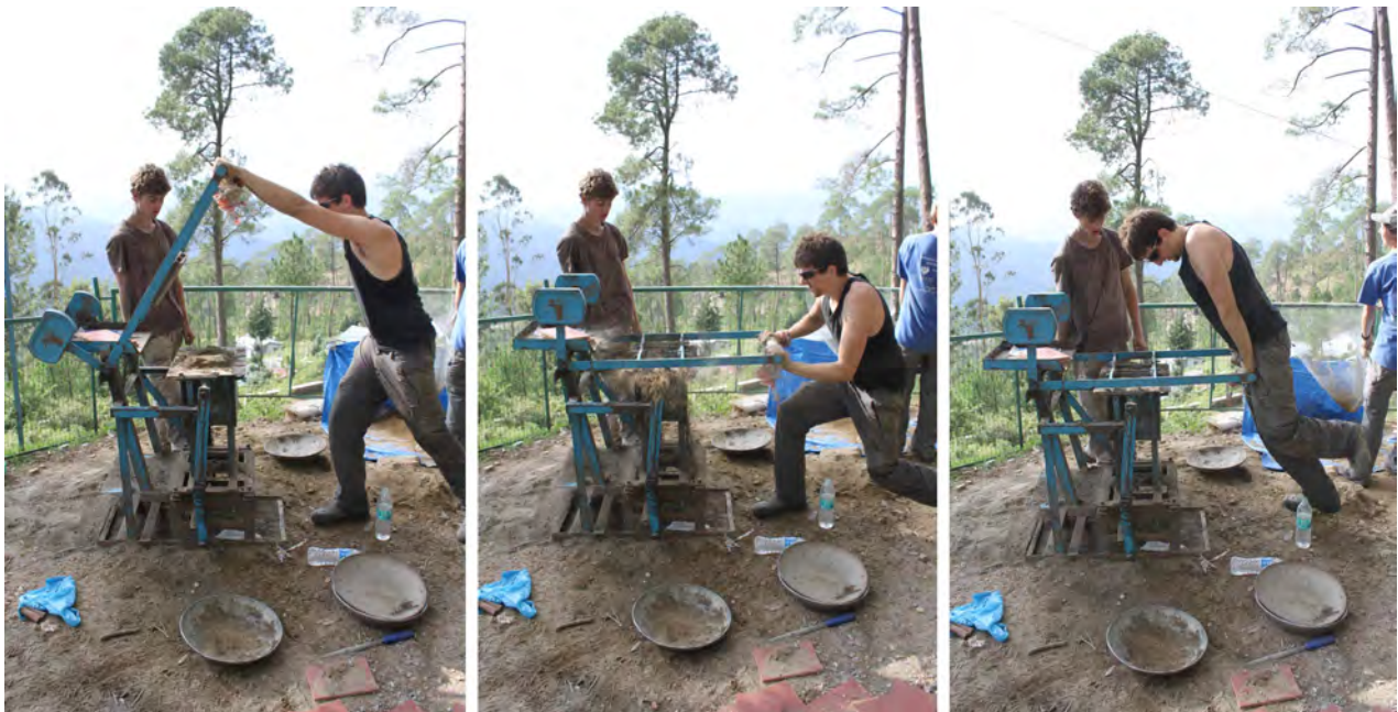
Figure 6: The manual block making machine (Source: Andrew Edwards).
