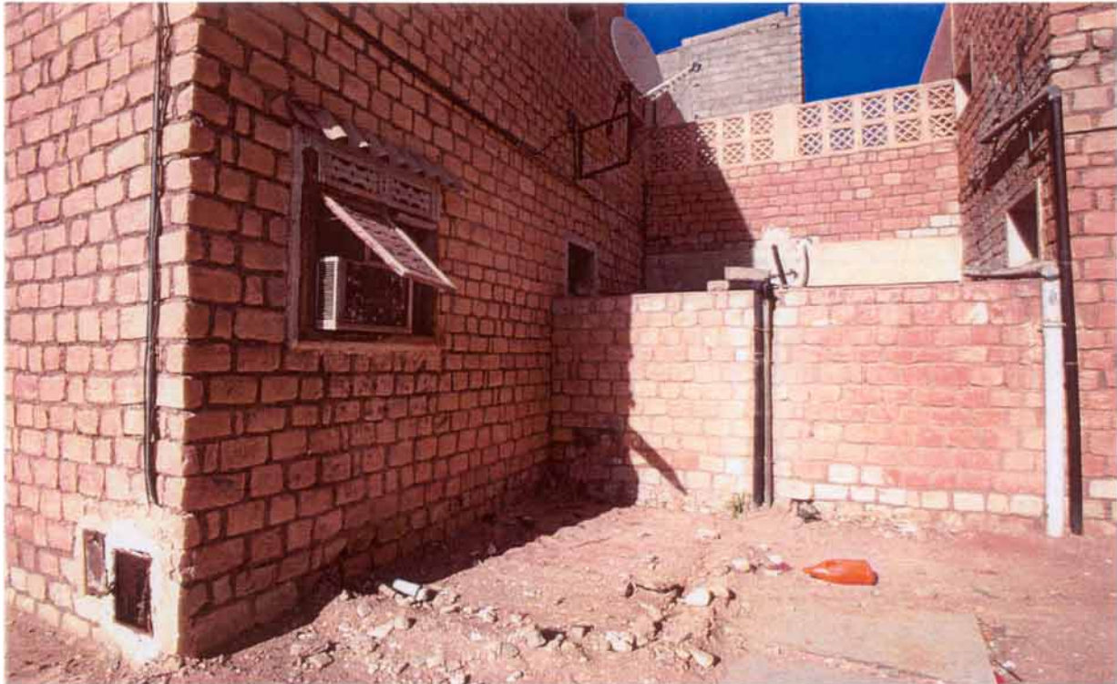
Above: The use of thick stone walls helped create cooler interiors. The staggered units and the close proximity of the clusters supplied the idea of developing hierarchical spaces and creating shaded walkways.
