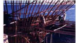
The mauuli is placed in horizontal layers, starting from the bottom to the top of the construction.
