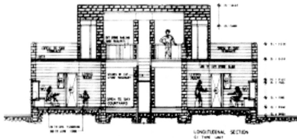
LONGITUDINAL SECTION A-TYPE UNIT
