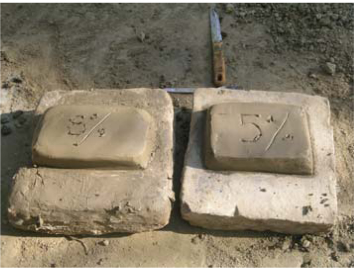
Trial tests of cement-stabilized local soil for durable and stronger plinth
