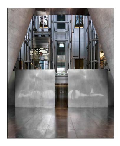
A rectangular structural core with elevators and utilities is placed slightly off-centre. It provides further structural support to the columns and allows for three-metre floor heights and open floor space.
