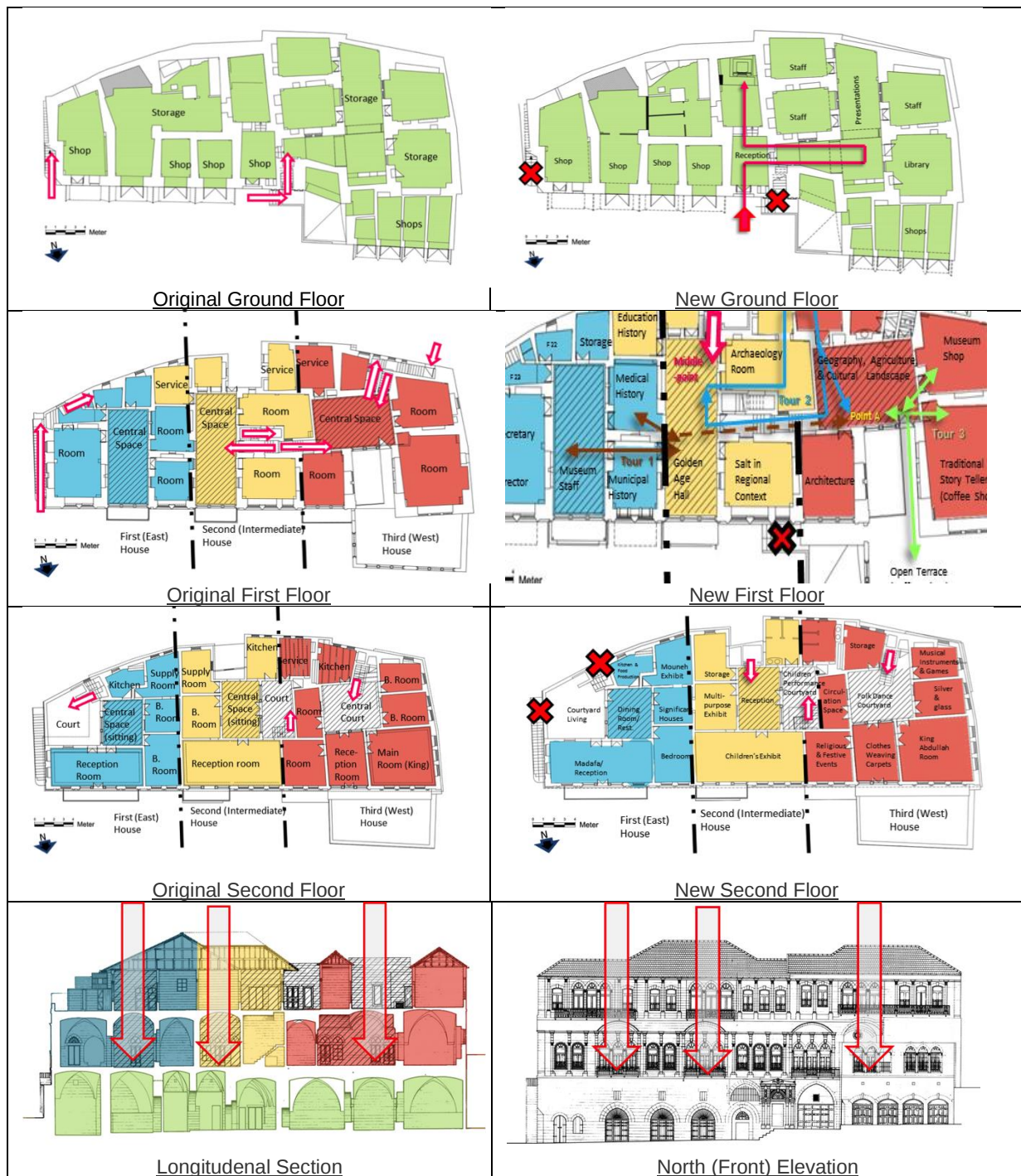
Figure 1. Drawings of the original houses and adaptive use (Source: Tiba Consultants, 2007; Redrawn by authors)
