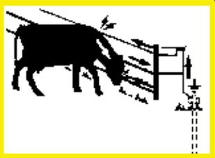
*Electric flow in Hot / Ground Wire Return fence is used in dry areas.*
