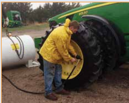
Travis Magary, with Mr. Tire in Ainsworth, injects Rim Guard, a non-corrosive and biodegradable liquid ballast.
