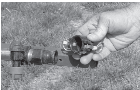
Figure 7. End cap on wet boom to drain and flush boom.
