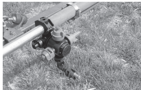
Figure 9. Multiple nozzle body on wet boom.
