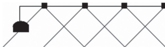
Figure 9. With a foam marker located one-half the distance between nozzles beyond the end nozzle, the marker is directly over the foam.
