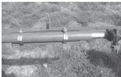
Figure 4. The bracket to hold the wet boom. The rubber hose protects the boom and the stainless steel hose clamps hold the wet boom in place.
