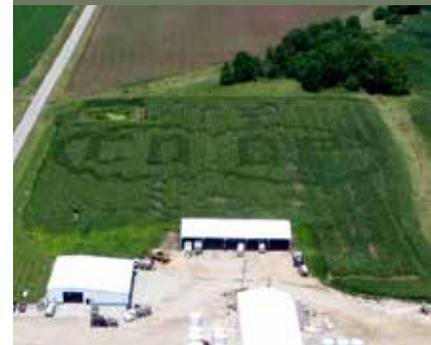
Pictured above is our Bellflower location. Notice on top of photo you can see the COOP logo in the corn field. This was done with our Multi-Hybrid Planter equipped with Precision Planting’s vSet Select corn meters. We used two different hybrids with different hues of green to show the affect and accuracy of the Multi-Hybrid technology.
