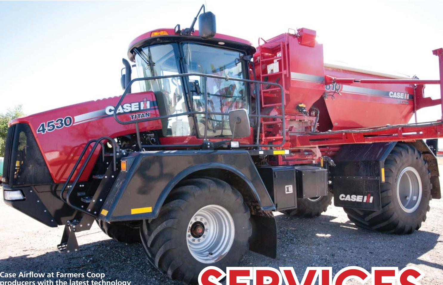
The new Case Airflow at Farmers Coop provides producers with the latest technology to apply fertilizer at variable rates.
