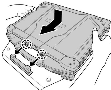
**Note:** Always remove the stylus before placing the Laptop PC onto the docking cradle.
