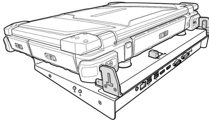
**Note:** The rear I/O door cannot be fully opened once the Laptop PC is fully secured to the docking cradle. If you need to access the COM port, it is recommended to use the COM port of the docking cradle.
