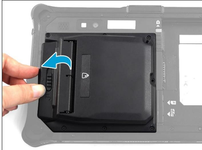
13. Slide the smart card reader lock switch to the lock position.
