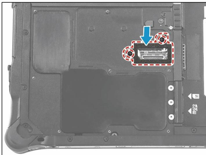
3. Connect the smart card reader harness to the mainboard connector.
