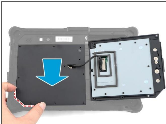
5. Attach the 3 screws to secure the smart card reader bracket to the lower case.
