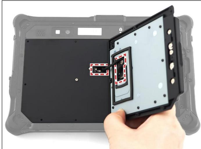
7. Align by the screw holes and then place the smart card reader on top of its bracket.
