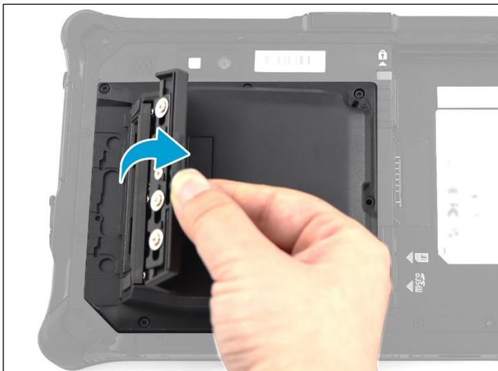
11. Attach the 2 screws to secure the smart card reader to the lower case.
