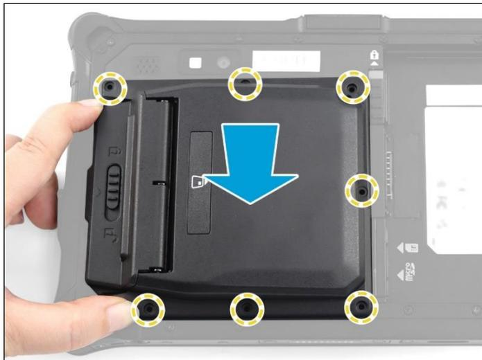
8. Attach the 6 screws to secure the smart card reader to the lower case.
