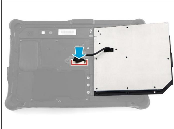
4. Place the smart card reader bracket onto its slot on the lower case. Make sure the cut edge of the bracket is aligned properly with the lower case.
