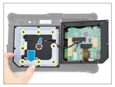
5. Fold the rear expansion module cable as shown in the image below.
