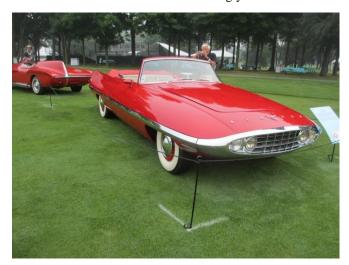
of drag of 0.17. Power went to the rear wheels through a Torque-Flite 3 speed transmission with push button controls.
