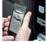
in the accident. This information allows a rescue to be performed with more safety for the responders and potentially faster for the vehicle occupants. Owners of cars without this feature can stop at any Mercedes dealer and have stickers generated for their vehicle.
