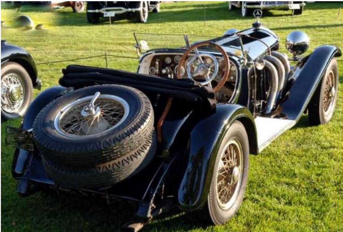
The external exhaust and twin rear mounted spares of a 1931 SSK, one of the ultimate sports cars of its day. Photo: harrysportcar.blogspot.com
