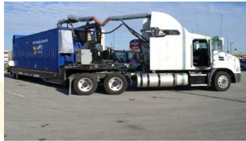
WVU Transportable Emissions Measurement System
