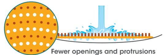
Fewer openings and protrusions cause pooling and creates splash
